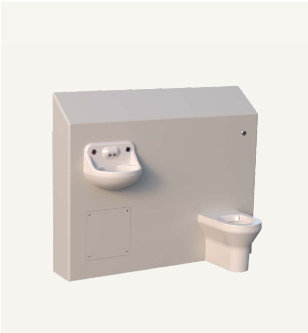
SANITATION DUCT LOW & HIGH LEVEL - RESIN Manufactured to meet the objectives and standards of an MOJ Safer Cell. A marine grade stainless steel or galvanised steel frame, finished with a mould and water-resilient substrate and solid surface resin material. When the surface is in contact with natural or artificial light its active properties allow air purification, elimination of harmful bacteria and ensures easy cleaning. Fire-resistant and ligature-resilient design with removable access panels using security-headed countersunk bolts. The dimensions and configuration of access panels are made to suit the specific requirements of a cell layout. Can be scribed to an uneven wall or floor surface without the need for skirting. All wall and floor junctions should be sealed with hard-setting epoxy non-pick mastic.
