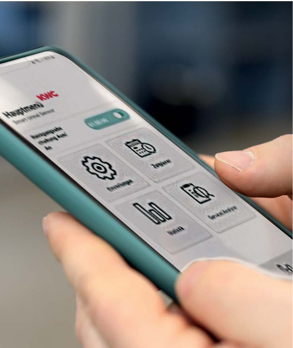
The "Smart Urinal" app is available for commissioning and controlling the Smart Urinal Sensor. It also enables other functions to be programmed.
