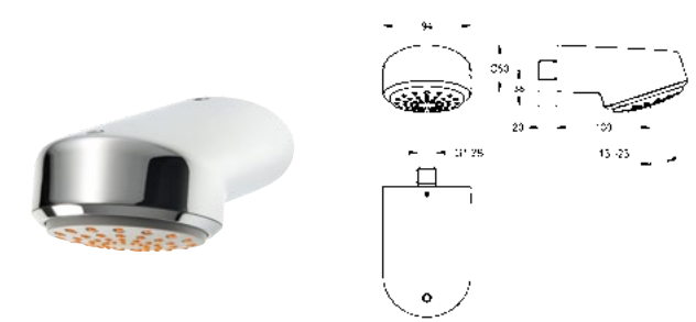
AQUAJET-COMFORT SHOWERHEAD FOR WALL CONNECTION AQUAJET-Comfort DN 15 showerhead with plastic jet face continuously adjustable between 13–23°, anti-limescale system and low aerosol formation. For wall connector with insertable connecting nozzle, diameter 26mm, high-polished chrome-plated brass housing, with integrated flow regulator 9.0l/min, ready for installation of anti-twist protection. Also suitable for shower trays, 800 x 800mm SHAC0013 Aquajet - comfort showerhead
