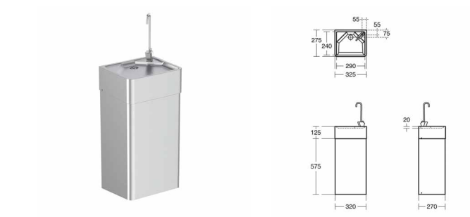
SISSONS DRINKING FOUNTAIN 700MM Junior height (700mm) floor mounted pedestal drinking fountain manufactured from stainless steel with a brushed finish. Designed with self closing valve with protected nozzle tominimise direct contact, complete with bottle filler. Tamper resistant pedestal Adult height 700mm Supplied with bottle Filler ANMX70
