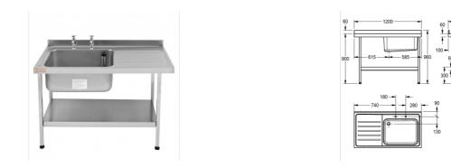
E20610L - Single bowl, LH single drainer. Midi sinks are manufactured from 1.2mm thick austenitic grade stainless steel polished to a satin finish. All sinks have two tapholes behind each bowl drilled at 180mm centres. Single bowl sinks are suitable for either 13mm pillar taps or mixer taps whereas the double bowl sinks are only suitable for pillar taps. Bowls are all supplied with 38mm waste and standpipe strainer overflow. An earthing lug is fitted under the drainer.
