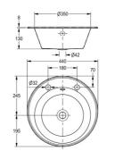
Washbasin for insetting into worktops, manufactured from grade 1.4301 (304) stainless steel - satin polish finish, material thickness 1.2mm. Prepared for 32mm waste outlet and verflow hole with two tapholes in the rear ledge behind the bowl - suitable for basin taps only (deck mixers cannot be fitted). Bowls are supplied complete with fixing clips for insetting into worktops.
