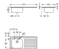
A single bowl/single drainer inset sink manufactured from 0.91 mm thick, austenitic type 304 stainless steel, satin polish finish. This sink has all four sides incorporating a rimmed edge profile, suitable for insetting into a standard sized worktop. The bowl is prepared for a 38 mm waste. Supplied complete with fixing clips.
