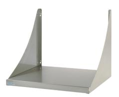
Wall mounted microwave shelf ideal for catering environments. Manufactured from 1.2 mm thick, grade 1.4301 (304) stainless steel with a satin polish finish. The triangular shaped wall brackets with 2 fixing holes are secured to the shelf using 2 nuts and bolts (supplied). The shelf can either be supported from underneath or hung from the brackets. A gap of 20 mm can be left behind the shelf to allow for cables. Fixing instructions supplied. Screws and plugs are not supplied.
