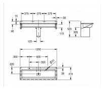
Wall mounted washtroughs with tap ledge and optional rear splashbacks incorporating manual or electronic self-closing water controls, manufactured from 1.2 mm thick stainless steel. 1200 mm Washtrough with tap ledge for 2 users.
