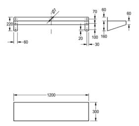
Manufactured from 1.2mm thick grade 1.4016 (430) stainless steel polished to a satin finish. All the shelves have integral triangular shaped wall brackets at each end. The brackets incorporate 2 fixing holes and together with the fixing holes provided in the upstand make for a strong and durable fastening to the wall. (Screws and plugs are not supplied). Ensure that the correct fixings are used to suit the type of wall. Additional loose fitting brackets are supplied for extra strength
