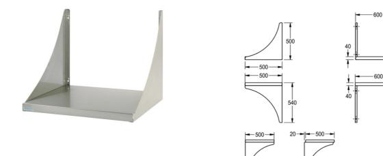
Manufactured from 1.2mm thick grade 1.4016 (430) stainless steel polished to a satin finish. All the shelves have integral triangular shaped all brackets at each end. The brackets incorporate 2 fixing holes and together with the fixing holes provided in the upstand make for a strong and durable fastening to the wall. (Screws and plugs are not supplied). Ensure that the correct fixings are used to suit the type of wall. Additional loose fitting brackets are supplied for extra strength
