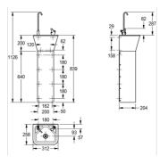
Drinking water fountains are manufactured from grade austenitic stainless steel, material thickness 1.2mm, supplied complete with 19mm waste and water bubbler. The wall mounted model is simply fixed to the wall using a joggle strip and integral mounting brackets. The pedestal version is fixed in the same way as the wall mounted version but incorporates extra fixing points within the pedestal support. No screws or wall plugs supplied.
