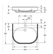
Single wash basin VARIUScare made of MIRANIT resin-bonded mineral material, with pore-free, smooth surface (temperature-resistant up to 80°C). Colour Alpine white. Wheelchair accessible and ergonomic designed based on the two-senses principle (tactile and visual), with integrated gripping edge and colour strip (RAL 7022). Seamless moulded bowl, without overflow. With tap hole, integral back panel with integrated brackets and holes for fixing. Rear contoured edge.
