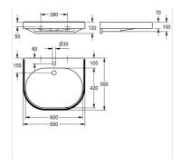
Single wash basin VARIUScare made of MIRANIT resin-bonded mineral material, with pore-free, smooth surface (temperatureresistant up to 80°C). Colour Alpine white. Wheelchair accessible and ergonomic designed based on the two-senses principle (tactile and visual), with integrated gripping edge and colour strip (RAL 7022). Seamless moulded bowl, without overflow. With tap hole, integral back panel with integrated brackets and holes for fixing. Rear contoured edge.
