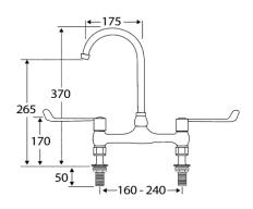
Lever operated mixer tap for connecting to hot and cold water. The mixer tap is supplied with 6" long levers which can be operated by either the elbows or wrists, using a quarter turn action. Suitable for use with tap holes between 165 - 240mm centres. Manufactured from chromium plated brass.
