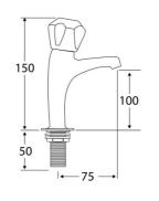
Pillar taps for connecting to hot and cold water. The 13mm pillar taps are manufactured from chromium plated brass and are complete with fluted handles which are moulded to give a comfortable and easy operation. Conforms to BS5412 standard.
