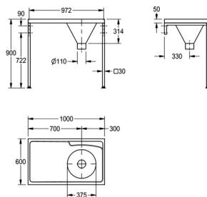
The unit should only be fed from a cistern or tank water supply. L or R after the code number refers to the handing of the drainer ie. left or right when facing front of unit. Unit can be mounted on either stainless steel cantilever brackets or Front leg supports give a working height of 900mm and have adjustable feet which can be screwed to the floor for extra stability.
