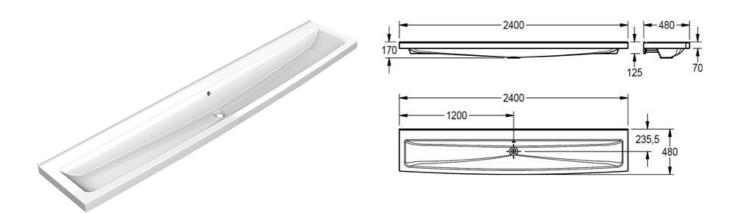
Miranit resin-bonded mineral material with smooth, pore-free surface (temperature resistant up to 80°C). Integral tap deck with integrated brackets and holes for fixing, mounting material, (hanger bolts and dowels), waste kit and mounting template included. No Tap holes (tap drill points marked underneath) with overflow, colour: Alpine white.
