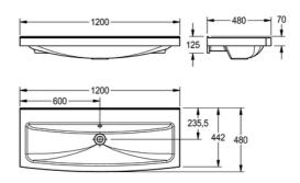
Washtrough made from Miranit resin bonded mineral material, with an alpine white gelcoat surface finish that's smooth, pore-free and temperature resistant up to 80°c. Washtroughs include a 32mm waste kit with overflow. Available with or without splashback, there is also a choice of either self-closing or electronic, touch free taps.
