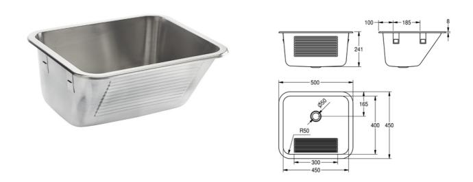
General purpose utility sink for inset mounting, stainless steel, surface satin finished, material thickness 0.9 mm, front panel with riffle, 1 1/2" flat perforated waste, incl. washer and clamps for inset mounting.
