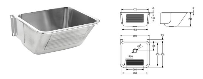
General purpose utility sink for wall mounting, stainless steel, surface satin finished, material thickness 0.9 mm, front panel with riffle, 1 1/2" flat perforated waste, prewelded mounting brackets.
