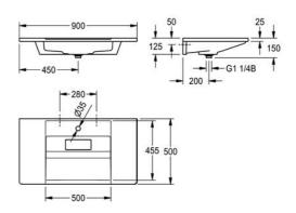
Single washbasin made of resin-bonded mineral composite, with pore-free, smooth gelcoat high-polished surface (temperature-resistant up to 80°C), with storage surfaces and integral back panel with integrated brackets for wall mounting. It has a seamless moulded bowl, no overflow and lowered tap ledge with tap hole. Mounting material and waste cover with lnoxPlus coating included.
