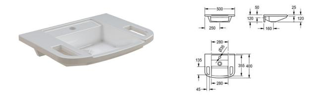
Hand washbasin, wheelchair accessible, made of resin-bonded mineral composite, with pore-free, smooth gelcoat high-polished surface (temperature-resistantup to 80°C), with integrated grab rails, storage surfaces and integral back panel with integrated brackets for wall mounting. It has a seamless moulded bowl, no overflow and lowered tap ledge with tap hole. Mounting material included.
