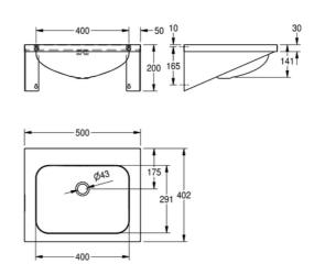
Single wash basin for wall mounting, stainless steel, surface satin finished, material thickness 1 mm, seamless welded bowl with diameter 500x400x200 mm, rectangular shape, 70 mm tap ledge, with overflow, 1 1/4" plug waste, drainage rewards centric, prewelded mounting brackets, incl. screws and dowels.
