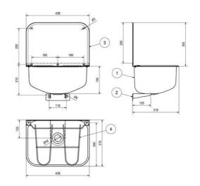
Wall Mounted cleaners sinkmanufactured from grade 1.4301 (304) stainless steel, material thickness 0.9mm, with splashback, hinged grating, 38mm BSP waste fitting and complete with integral wall bracket.
