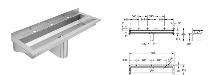
Wall mounted washtroughs with tap deck and optional rear splashbacks incorporating manual or electronic self-closing water controls, manufactured from 1.2mm thick stainless steel. 1800mm Washtrough with Tap Deck for 3 users
