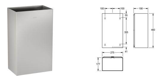
Waste bin for wall mounting, stainless steel, surface satin finished, material thickness 0.8 mm, rounded edges, mounting either with mounting bracket or directly onto the wall, incl. stainless steel screws and dowels.
