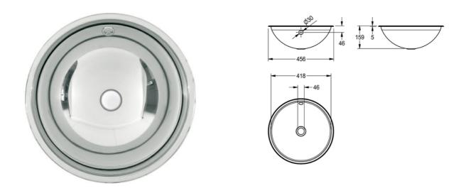
Round inset vanity basin, can be mounted from top or underneath, stainless steel, material thickness 1 mm, bowl diameter 418 mm, with overflow, incl. 5/4" overflow kit without waste, stainless steel lugs for underneath mounting are included. Outcut diameter for mounting from top: 436 mm, outcut diameter for mounting from underneath: 410 mm
