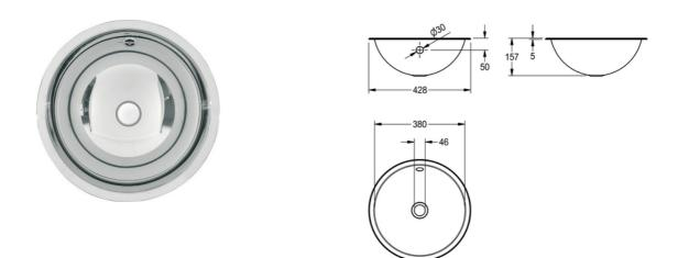
Round inset vanity basin, can be mounted from top or underneath, stainless steel, material thickness 1 mm, bowl diameter 380 mm, with overflow, incl. 5/4" overflow kit without waste, stainless steel lugs for underneath mounting are included. Outcut diameter for mounting from top: 408 mm, outcut diameter for mounting from underneath: 370 mm
