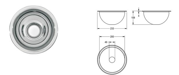
Round inset vanity basin, can be mounted from top or underneath, stainless steel, material thickness 1 mm, bowl diameter 200 mm, without overflow, incl. 5/4" flat perforated and plug waste, stainless steel lugs for underneath mounting are included. Outcut diameter for mounting from top: 212 mm, outcut diameter for mounting from underneath: 190 mm
