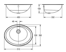
Round inset vanity basin, can be mounted from top or underneath, stainless steel, material thickness 1 mm, bowl diameter 450x330 mm, with overflow, incl. 5/4" overflow kit without waste, stainless steel lugs for underneath mounting are included.
