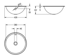
Round inset vanity basin, can be mounted from top or underneath, stainless steel, material thickness 1 mm, bowl diameter 380 mm, with overflow, incl. 5/4" overflow kit without waste, stainless steel lugs for underneath mounting are included. Outcut diameter for mounting from top: 408 mm, outcut diameter for mounting from underneath: 370 mm
