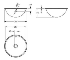
Round inset vanity basin, can be mounted from top or underneath, stainless steel, material thickness 1 mm, bowl diameter 357 mm, with overflow, incl. 5/4" overflow kit without waste, stainless steel lugs for underneath mounting are included. Outcut diameter for mounting from top: 368 mm, outcut diameter for mounting from underneath: 350 mm
