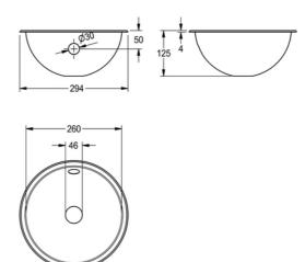
Round inset vanity basin, can be mounted from top or underneath, stainless steel, material thickness 1 mm, bowl diameter 260 mm, with overflow, incl. 5/4" overflow kit without waste, stainless steel lugs for underneath mounting are included. Outcut diameter for mounting from top: 274 mm, outcut diameter for mounting from underneath: 250 mm
