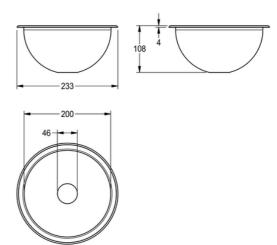
Round inset vanity basin, can be mounted from top or underneath, stainless steel, material thickness 1 mm, bowl diameter 200 mm, without overflow, incl. 5/4" flat perforated and plug waste, stainless steel lugs for underneath mounting are included. Outcut diameter for mounting from top: 212 mm, outcut diameter for mounting from underneath: 190 mm
