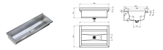
PLANOX seamless welded washtrough for wall mounting, chromium nickel steel, satin finished surface, material thickness of washtrough 0.8 mm / side panels 1.2 mm, side panels with integrated wall brackets, without tap ledge or overflow, 40 mm rear upstand, central waste. Supplied with 38mm dome waste and mounting materials. For a length of 1800 mm or more, an additional bracket is supplied. Optional shroud and splashback are available as extras. Special lengths are available on request.
