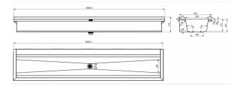
PLANOX seamless welded washtrough for wall mounting, chromium nickel steel, satin finished surface, material thickness of washtrough 0.8 mm / side panels 1.2 mm, side panels with integrated wall brackets, without tap ledge or overflow, 40 mm rear upstand, central waste. Supplied with 38mm dome waste and mounting materials. For a length of 1800 mm or more, an additional bracket is supplied. Optional shroud and splashback are available as extras. Special lengths are available on request
