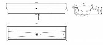
PLANOX seamless welded washtrough for wall mounting, chromium nickel steel, satin finished surface, material thickness of washtrough 0.8 mm / side panels 1.2 mm, side panels with integrated wall brackets, without tap ledge or overflow, 40 mm rear upstand, central waste. Supplied with 38mm dome waste and mounting materials. For a length of 1800 mm or more, an additional bracket is supplied. Optional shroud and splashback are available as extras. Special lengths are available on request.
