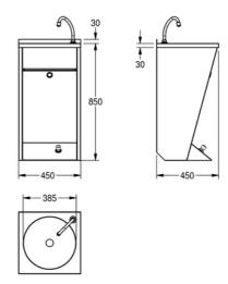
Single wash basin for floor or wall mounting, stainless steel, surface satin finished, material thickness 1 mm, seamless welded round bowl with diameter 380 mm, rectangular shape, 35 mm tap ledge, without overflow, 1 1/4" plug waste, drainage centric, incl. premounted spout, floor standing trap cover with premounted self-closing valve for foot operation, water temperature adjustable with valve, front cover can be removed, incl. screws and dowels.
