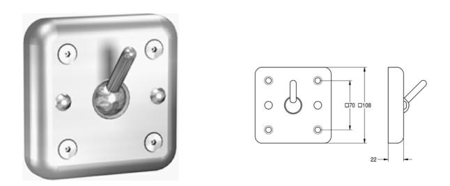
Coat hook, stainless steel, material thickness 2 mm, visible surface satin finished. Safety hook tilts downwards when overloaded, projection 30 mm from wall plate. Dimensions  $108 \times 108 \times 52$  mm (W x H x D).
