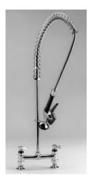
Manufactured from chromium plated brass, both are suited for those locations where there is a need for a thorough rinsing of utensils and crockery in dishwashing areas. F1061 monobloc spray is designed to be fitted into a single taphole behind the bowl whereas the F1062 deck mixer spray fits into taphole centres of 180mm. Both models are supplied complete with spray valve and 150mm wall bracket. Suitable for temperatures up to 130°F.
