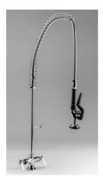
Manufactured from chromium plated brass both the pre-rinse overhead sprays are suited for those locations where there is a need for athorough rinsing of utensils and crockery in dishwashing areas. F1061 monobloc spray is designed to be fitted into a single taphole behind the bowl whereas the F1062 deck mixer spray fits into taphole centres of 180mm. Both models are supplied complete with spray valve and 150mm wall bracket. Suitable for temperatures up to 130°F. WRAS approved
