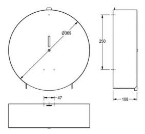
Jumbo roll holder for wall mounting, stainless steel, surface satin finished, material thickness 0.9 mm, closed round casing with inspection window, paper withdrawal over two tear-off edges, locked with hexagonal allen screw, for 1 roll with max. Ø 350 mm, incl. stainless steel screws, dowels and hexagonal allen key.
