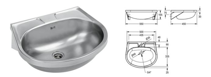
Single wash basin for wall mounting, stainless steel, surface satin finished, material thickness 1 mm, seamless welded bowl with diameter 500x335x155 mm, oval shape, 90 mm tap ledge, prewelded mounting brackets, with soap dish, incl. screws and dowels.
