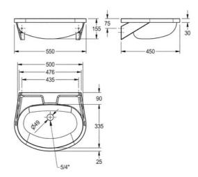
Single wash basin for wall mounting, stainless steel, surface satin finished, material thickness 1 mm, seamless welded bowl with diameter 500x335x155 mm, oval shape, 90 mm tap ledge, prewelded mounting brackets, with soap dish, incl. screws and dowels.
