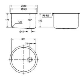
Round inset basin, can be mounted from top or underneath, stainless steel, surface high polished, material thickness 1 mm, bowl diameter 300 mm, without overflow, incl. 5/4" flat perforated waste, stainless steel lugs for underneath mounting are included.
