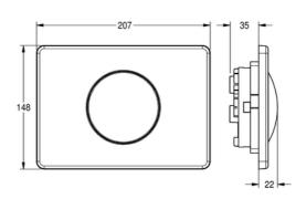
Flushing plate for wall-installation cistern, operation from front, consisting of operating button, button mounting, installation frame, fixing bolts and securing screw, made of stainless steel, dimensions 207x148 mm (WxH).
