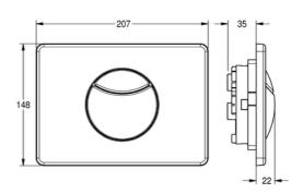
Flushing plate for wall-installation cistern, operation from front, 2-level flushing or start/stop flushing, consisting of operating button, button mounting, installation frame, fixing bolts and securing screw, dimensions 207 x 148 mm (W x H).
