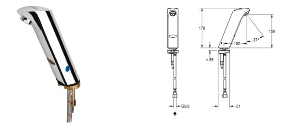
PROTRONIC-S battery-supplied washbasin tap with touch-free operation, DN 15 with aerator and integrated flow control, for connection to pre-mixed warm or cold water supply, polished chromium-plated brass, 6 V battery. WRAS approved.
