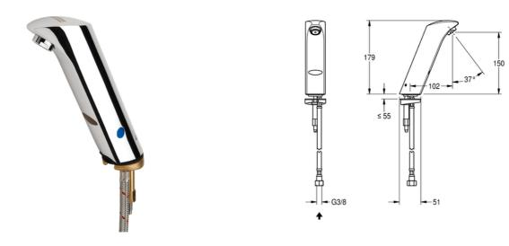
PROTRONIC-S battery-supplied washbasin tap with touch-free operation, DN 15 with aerator and integrated flow control, for connection to pre-mixed warm or cold water supply, polished chromium-plated brass, 6 V battery. WRAS approved.
